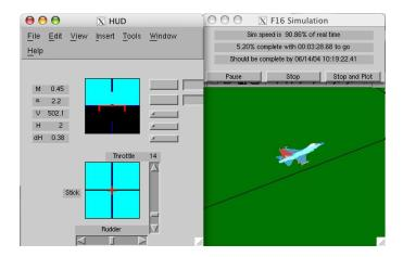
The simulation function also will automatically linearize the nonlinear dynamics and generate a state space model. In addition, a trimming algorithm is included which can trim the aircraft in a variety of flight modes.
