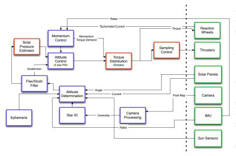
attitude control and actuation distribution are provided in separate modules, as illustrated in the example of an attitude control system implemented in AAVC (left).
