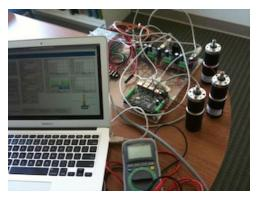
connected to a ControlDeck controller. The laptop shows the VisualCommander drag and drop graphical interface displaying data from the motors, which are part of a 3-axis gimbal mechanism for CubeSat testing.
