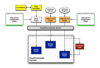
ControlDeck is used to write flight software and DSim to write simulation models. The ControlDeck libraries implement complete control systems for atmospheric vehicles and spacecraft. Whereas, the DSim modules are for a wide variety of spacecraft and aircraft hardware, dynamical models and environmental models.
